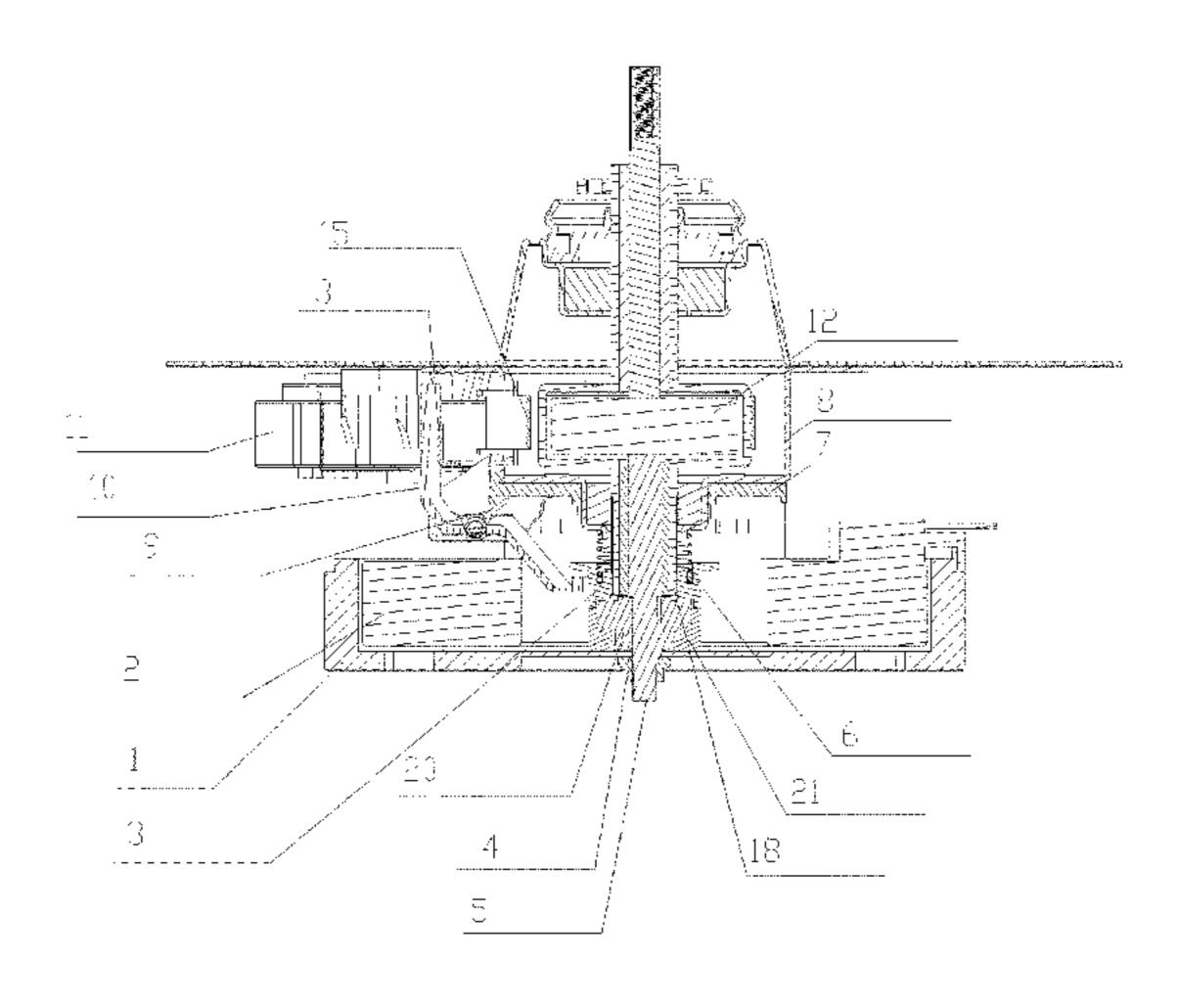
braking belt (15) and the clutch shaft sleeve (3) are separately connected to a traction motor (11) by means of a control apparatus.
