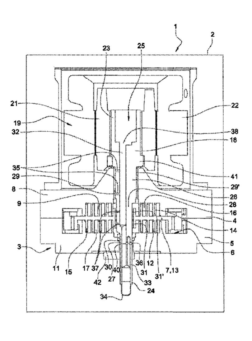
the first and second guide bearings (29, 30) being located on either side of the orbiting scroll arrangement (7).
