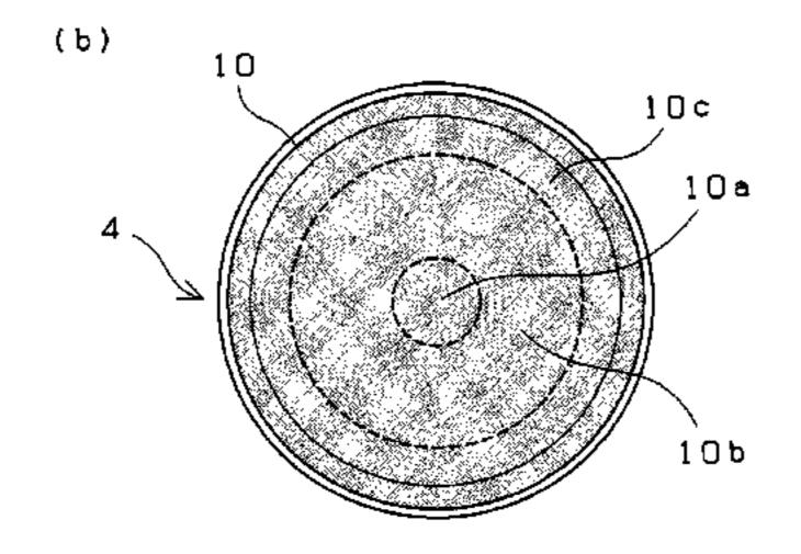
thickness is larger than that of each of the central part (10a) and the outer edge part (10c) is formed inside the intermediate part (10a).
