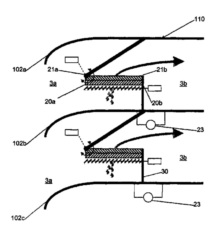
actuatable to co-operate with the bypass element for isolating the water separator from the air mass when the bypass element is in the second closed position.
