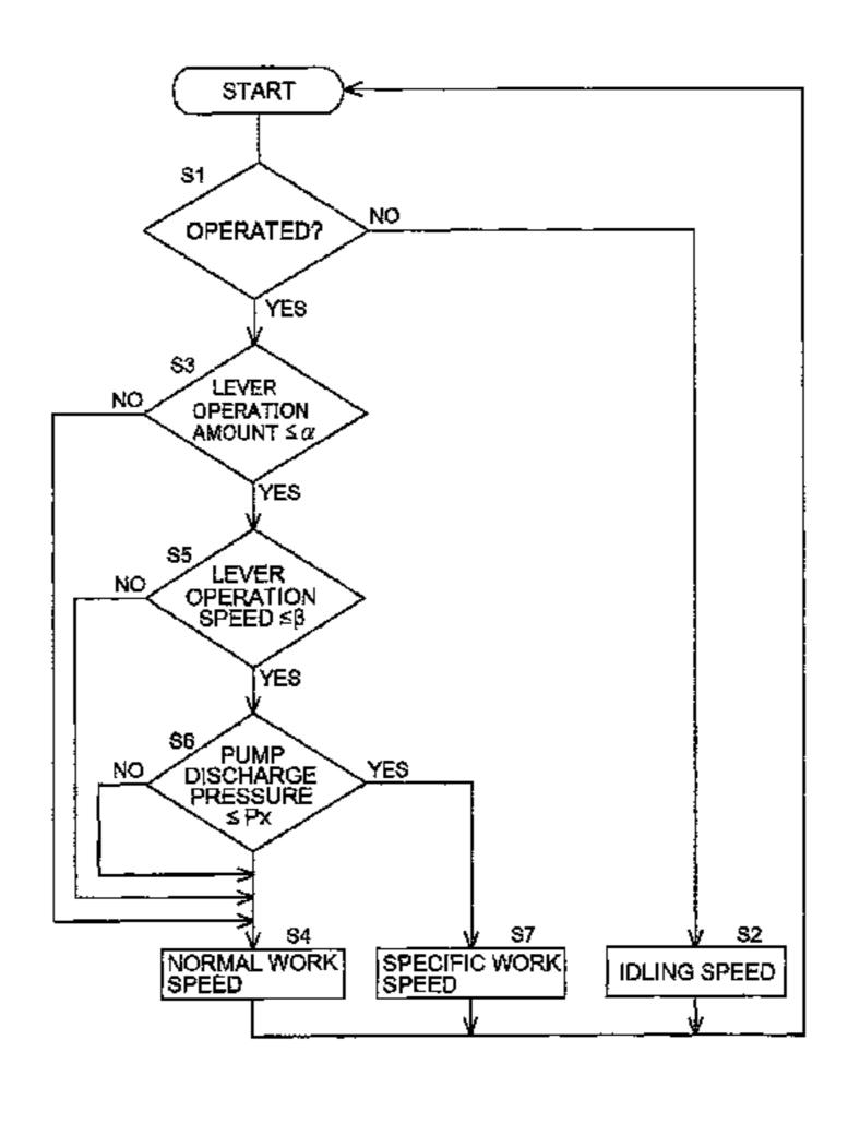
higher than the idling speed but lower than the normal work speed, on detecting execution of the specific work which is performed with an operation amount of the operating device such as a boom operating device (16) being kept small in a state in which the speed of the engine (11) is kept at the idling speed.
