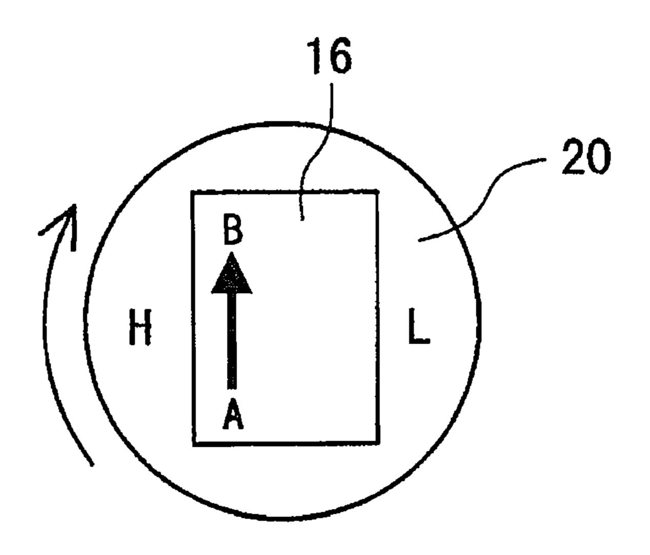
slide starting point toward the high cam terminating point along the slope of the cam sliding contact surface, the valve lifter is not subjected to a force around the reciprocating axis from the cam and therefore, the direction of the valve lifter is maintained constant.
