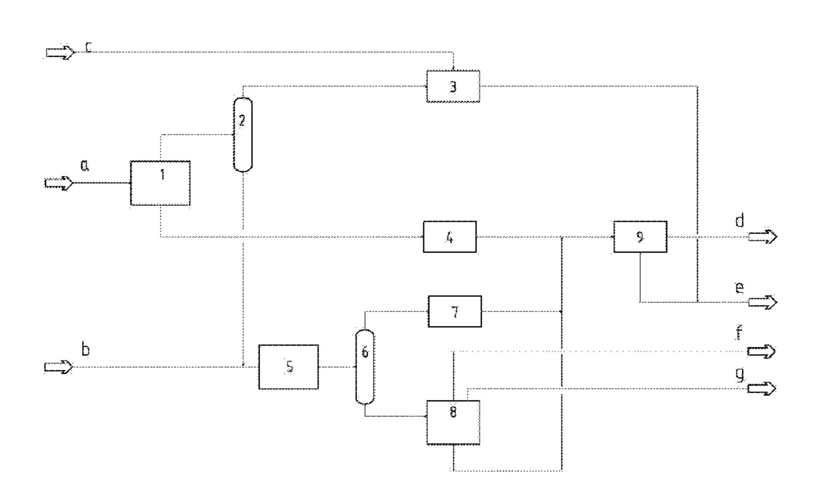
increased by introducing the reforming patent technology. The sulfur content in gasoline products is lowered to 10 ppm by selecting the device and method. The device and method have obvious advantages in investment, hydrogenation scale, product cleanliness, quality, etc.
