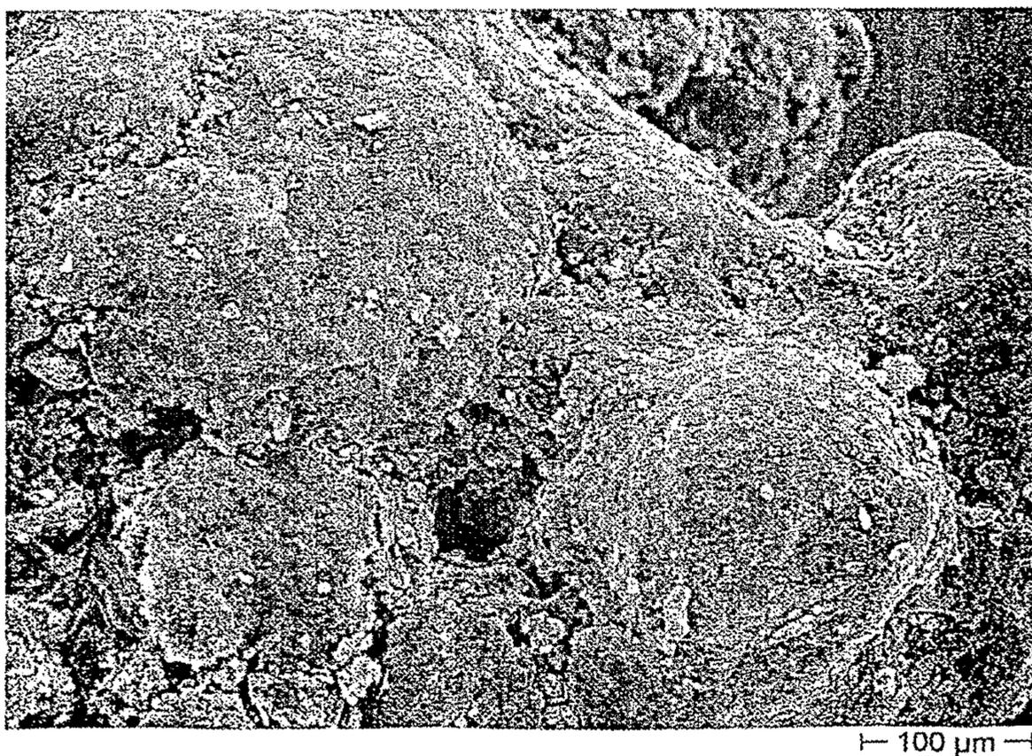
Figure 13A: Surface of Nal-Extr granulates at 30x magnification. The voltage was 10 kV. The bar length corresponds to 1 mm.
