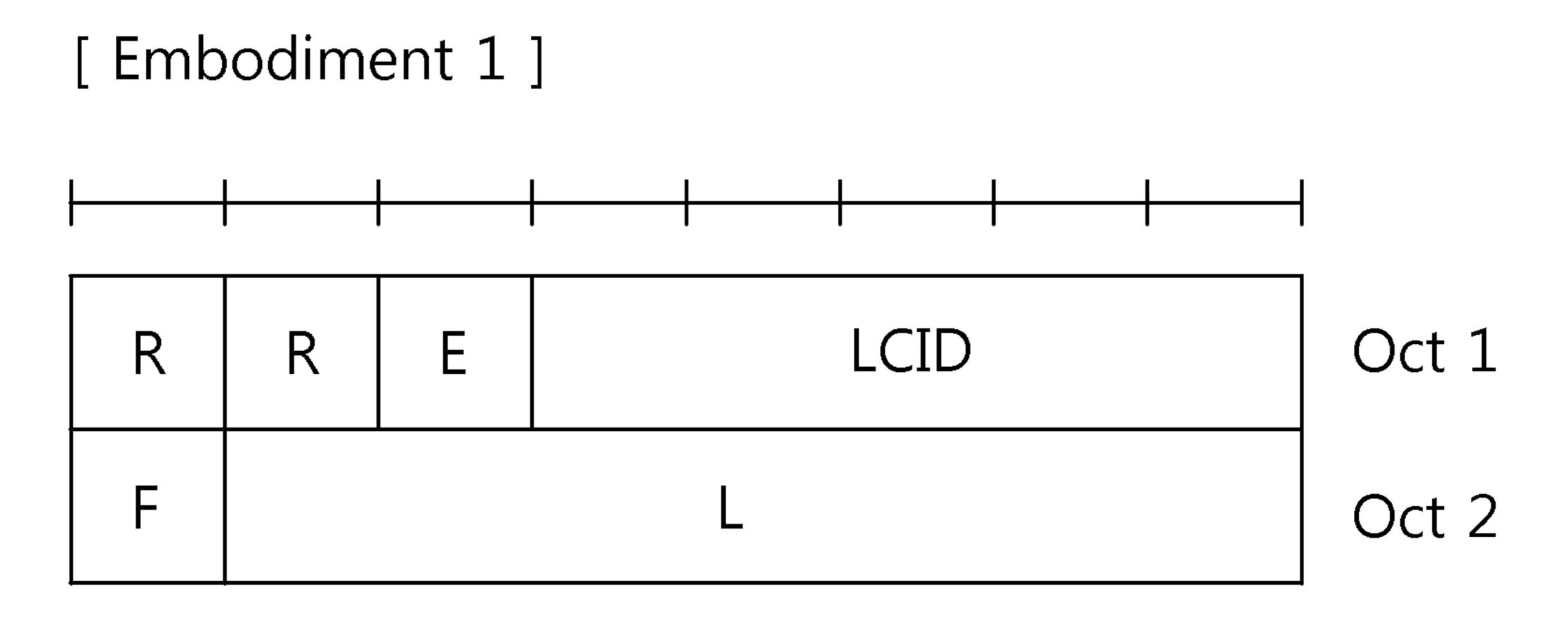
R/R/E/LCID/F/L sub-header with 7-bit L field
