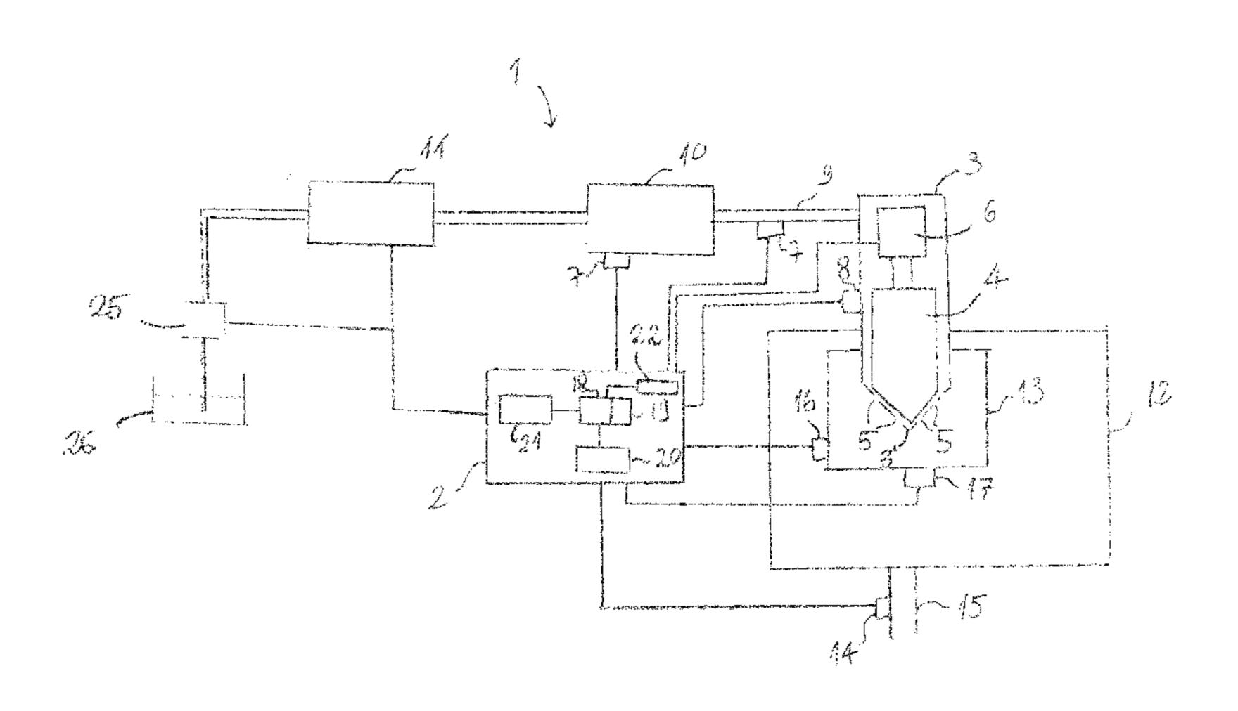
in at least one of the subsequent injection cycles as a function of a deviation of the actual stroke height from the target stroke height.
