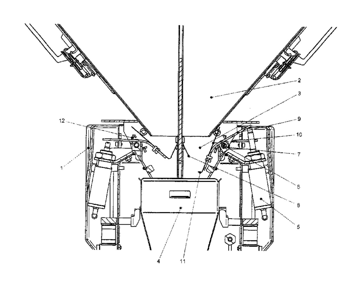
valve (3), in particular as a flap-type metering valve. The metering valve (3) consists of a part, a closure (7), movable via a horizontal axis (6) and a fixed part, a scraper (8). The movable part has an operating arm (9) for an actuator (5) and at the end facing towards the fixed part has a closure plate (10) having a scraper projection (11). In the closed state of the metering valve (3) the scraper projection (11) touches the scraper (8).
