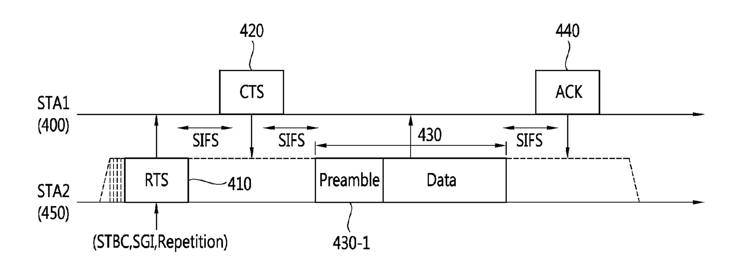
transmission efficiency by adaptively determining a transmission mode of a PCLP header to a channel situation.
