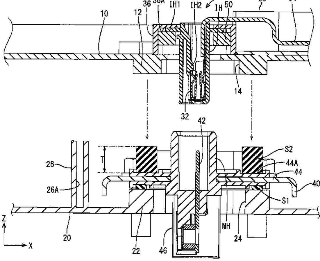
the inverter case 10 and the motor side terminal block 40 to surround a connection portion of the inverter side terminal 32 and the motor side terminal 42 and configured to seal a space between the inverter case 10 and the motor side terminal block 40.
