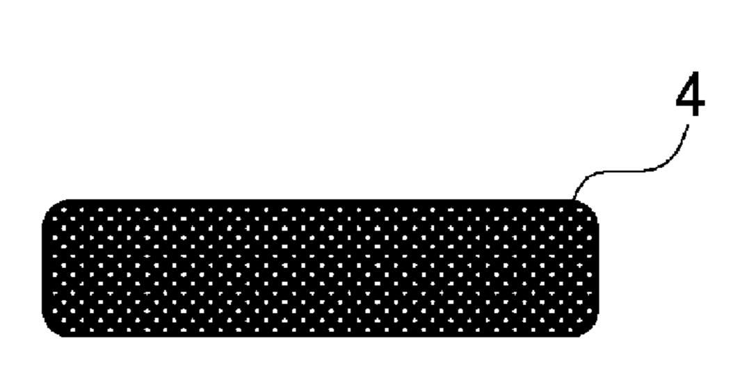
in the ion-injection region (3). This method is characterized in that the orientation of the sapphire substrate (4) is a C-plane having an off-angle of 1 degree or less.
