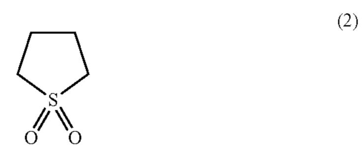
The lower limit of the sulfolane content of the organic solvent is preferably 10% by mass, and the upper limit thereof is preferably 90% by mass. If the sulfolane content is less than 10% by mass, the electrolyte may become less soluble. If the sulfolane content is more than 90% by mass, the coagulation point of the electrolyte solution may rise. The lower limit of the sulfolane content is more preferably 20% by mass, and the upper limit thereof is more preferably 80% by mass.
