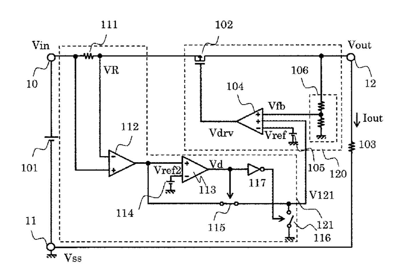
thereby switch control of the output transistor from control based on the constant voltage control circuit to control based on the overcurrent protective circuit.
