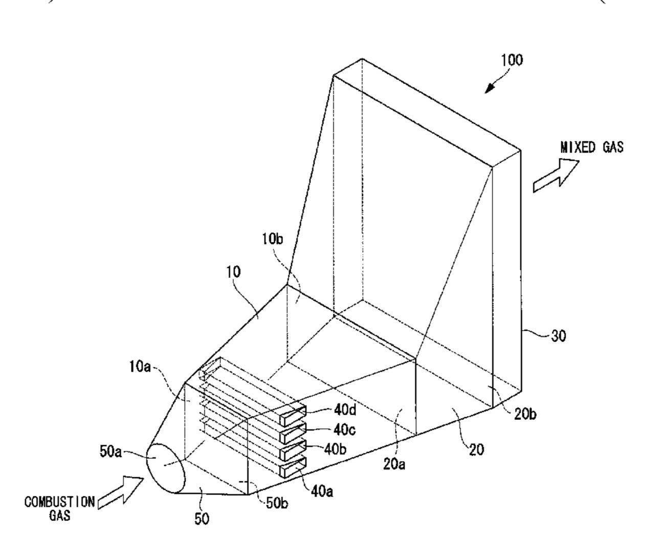
of the flow inlet and the flow outlet with respect to the passage length of the mixing duct is smaller than a difference of maximum dimensions in the width direction of the flow inlet and the flow outlet with respect to the passage length of the expanded duct.
