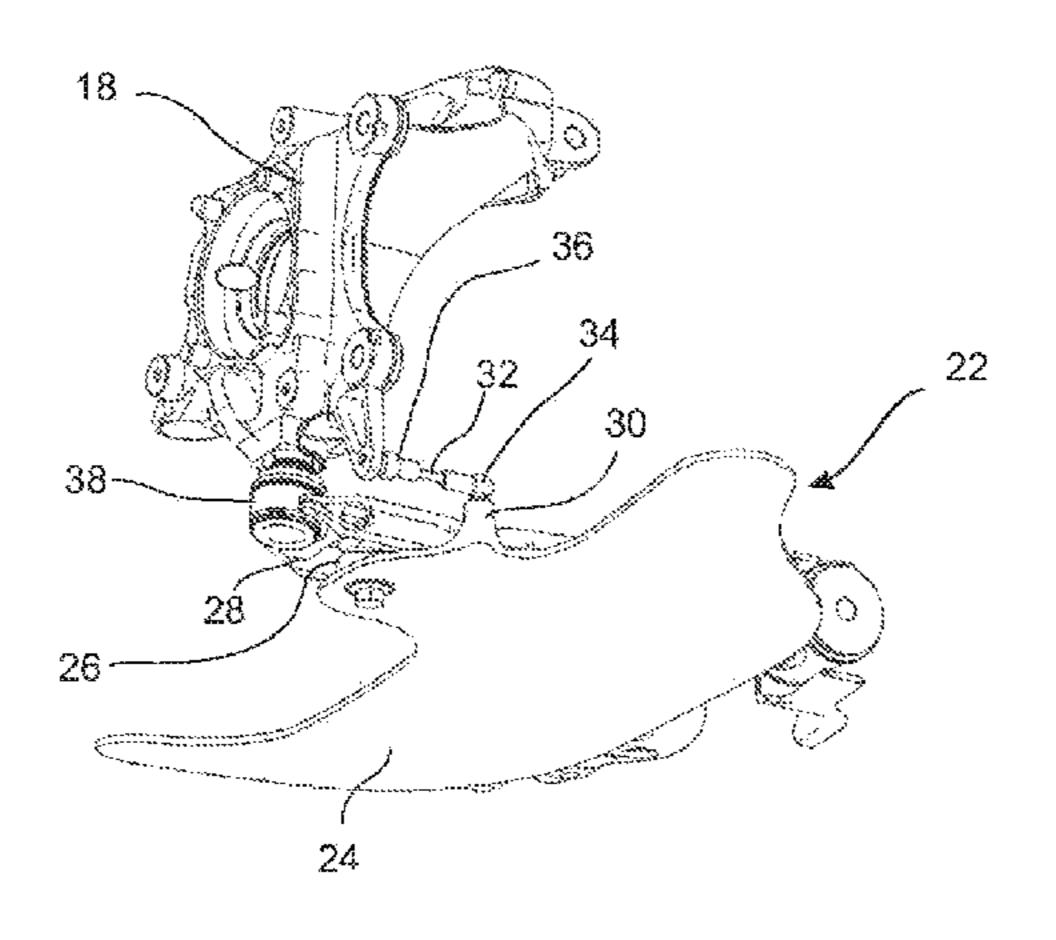
mounting point when the wheel carrier is pivoted. A subassembly having the underbody panelling part is also provided.
