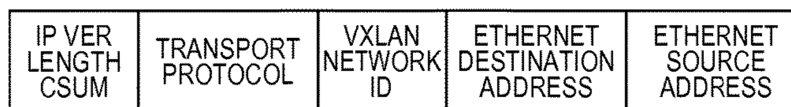
ONE SET OF HEADER INFORMATION READ OUT OF THE FIRST EGRESS PACKET MODIFIER MEMORY
