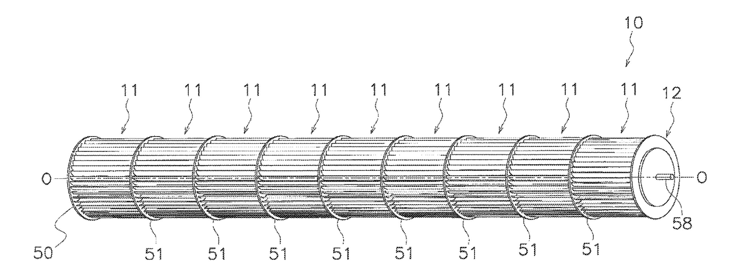
maximum thickness is located 40% to 60% from the inner peripheral side arc in the lengthwise direction. The blades are disposed such that the inner peripheral side arcs are positioned on an inner peripheral side of the support plate and the outer peripheral side arcs are positioned on an outer peripheral side of the support plate. A flow path width between the plurality of blades gradually decreases from the inner peripheral side toward the outer peripheral side of the support plate.
