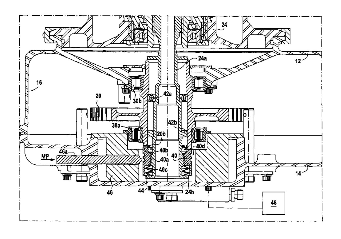
movement of a plunger pin having one end co-operating with an outer helical groove in the dog clutch.
