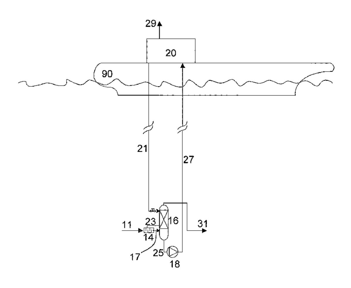
topside regeneration involving adding pressurized hot natural gas to the treatment fluid subsea as a lift gas and separating the natural gas from the treatment fluid topside before the treatment fluid enters the treatment unit is described.
