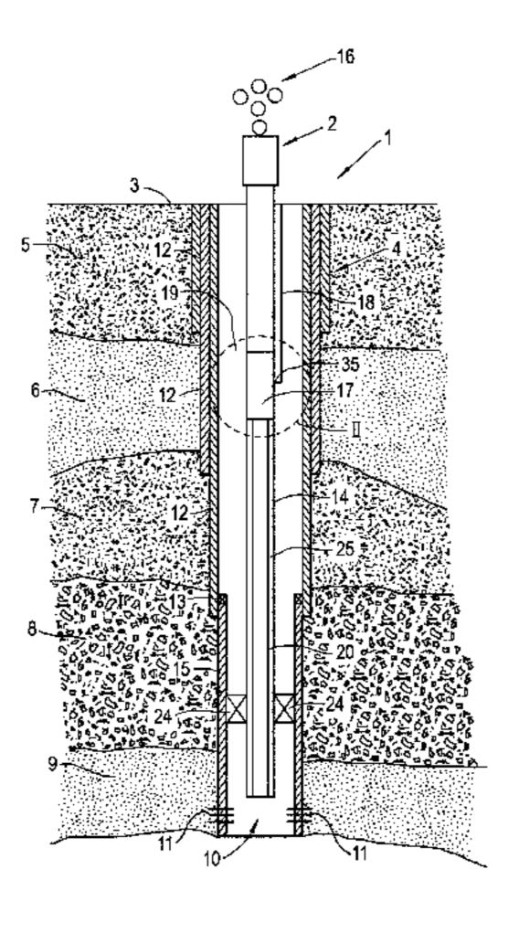
stream, and controlling the flow of gas from the annulus between the outer wall of the velocity string and the inner wall of the production tubing to the primary gas stream by means of the control valve wherein a controlled mass flow of said gas is combined with the primary gas stream.
