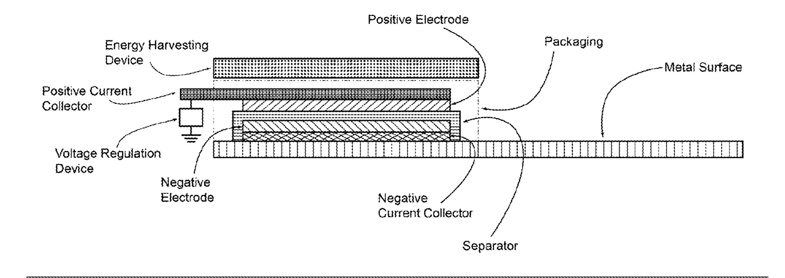
composition above the positive electrode layer to form a positive electrode current collector layer above the positive electrode layer.
