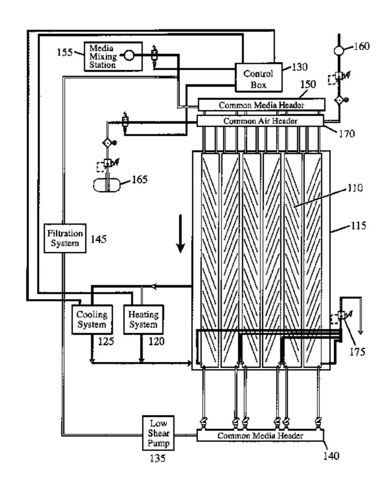
prises gas exchange, temperature control, air pumping, liquid pumping, filtration, media recycling and harvesting methods. For biofuels production, the photobioreactor system can comprise a separate growth photobioreactor and secondary stress reactor.
