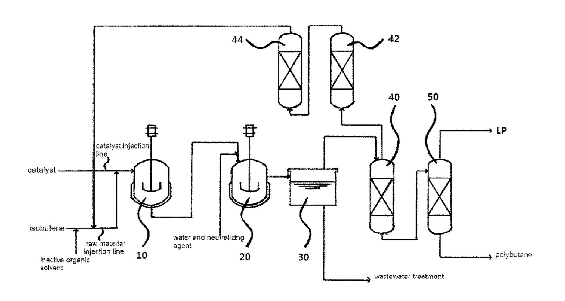
neutralizing/washing tank for removing the catalyst from the reaction product and neutralizing the reaction product; a separation tank for separating the reaction product into organic compounds and water; a C4 distillation column for distilling an unreacted raw material and the inactive organic solvent from the organic compounds; and an impurity adsorption column for removing halogen acid from the distilled unreacted raw material and the inactive organic solvent using an adsorbent.
