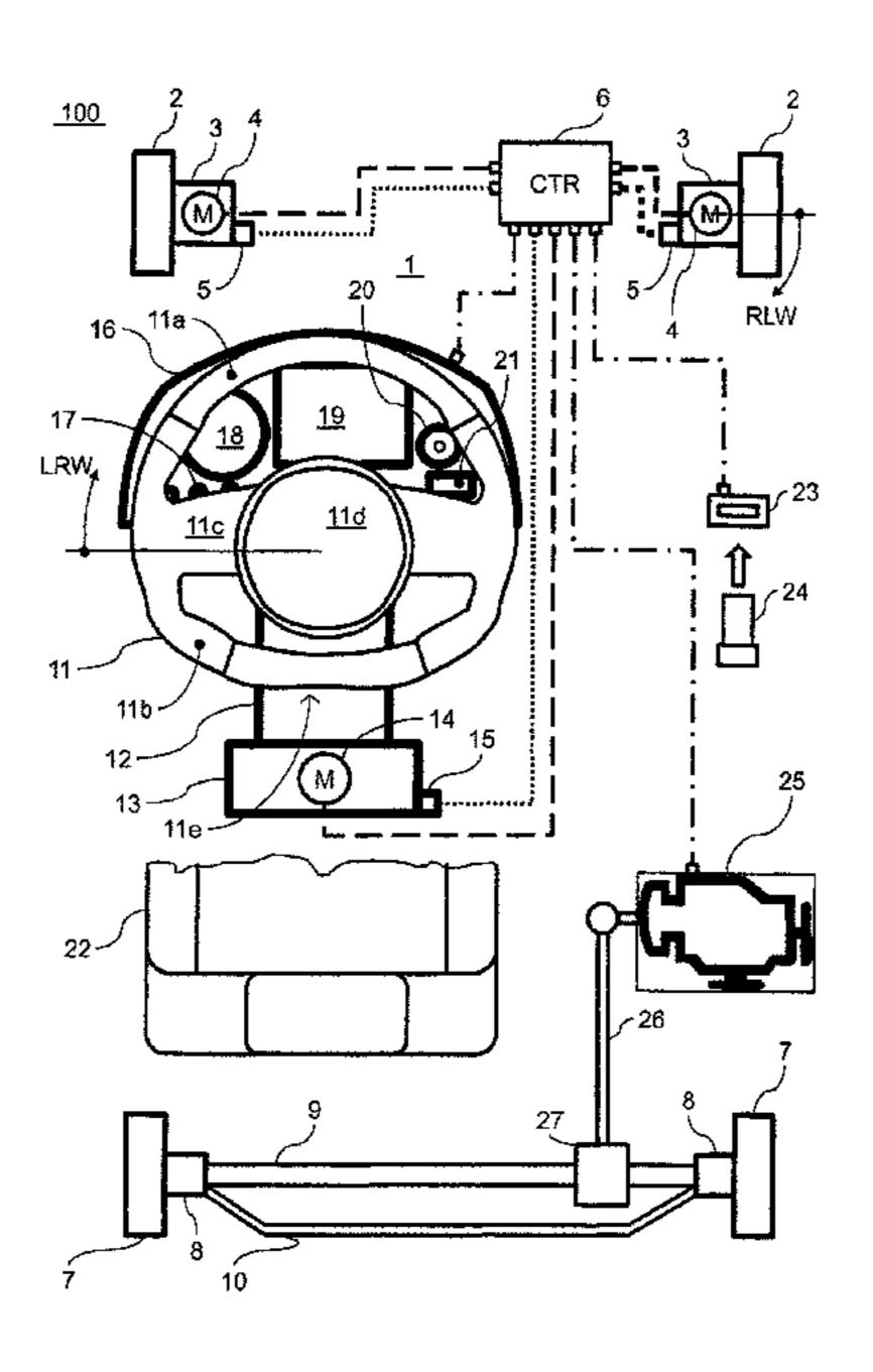
steerable wheel, and a controller for controlling the wheel steering drive and the steering wheel actuator. When the ignition is switched off, the steering wheel is moved with the steering wheel actuator automatically into a neutral position that is independent of a wheel angle of the steerable wheel.
