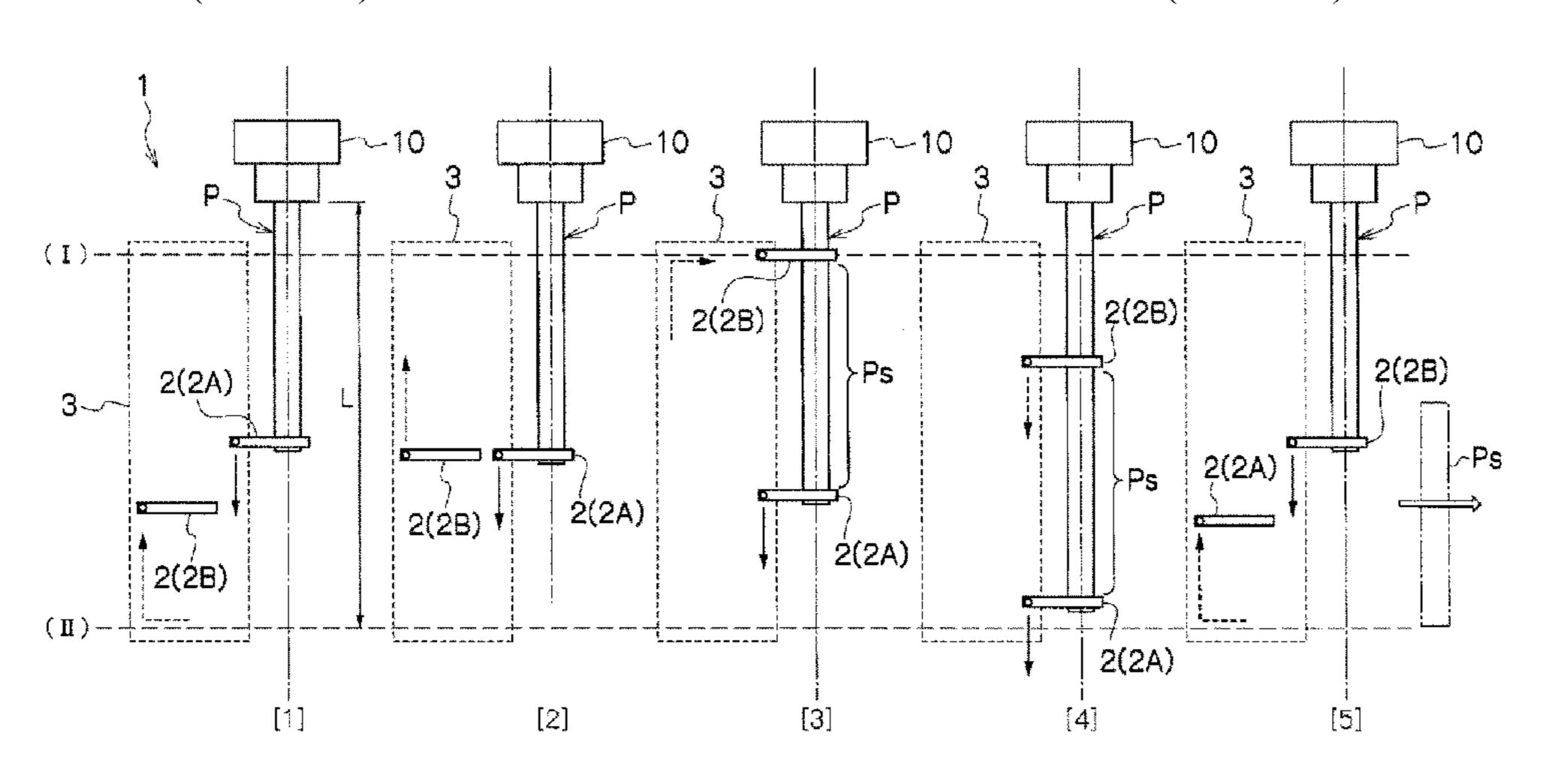
position near the extrusion die and moving to a second position separated from the extrusion die such that, before the preceding tension chuck is separated by a set distance from the extrusion die at the second position, the following tension chuck grasps the parison at the first position, and then the parison section is supplied to the blow molding die.
