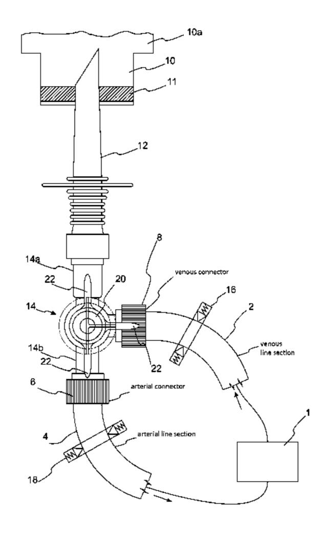
which is arranged directly downstream of the universal medical fluid container. A conduit of the 3-way switch is preferably coupled with a spike or a similar connecting device or is formed in one piece together with it.
