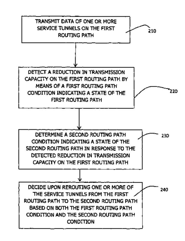
determined indicating a state of the second routing path (134) in response to the detected reduction in transmission capacity on the first routing path (132). It is decided upon rerouting one or more of the service tunnels from the first routing path (132) to the second routing path (132) based on both the first routing path condition and the second routing path condition.
