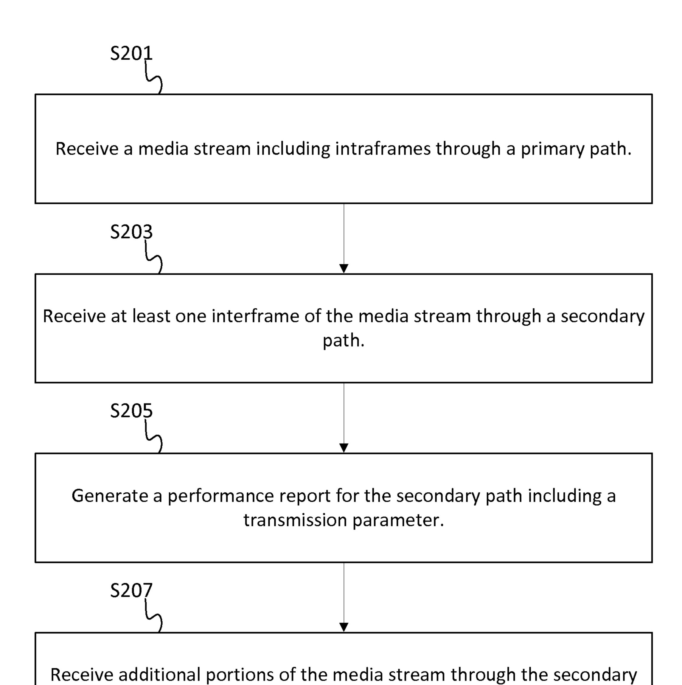
path when the transmission parameter exceeds a threshold value.
