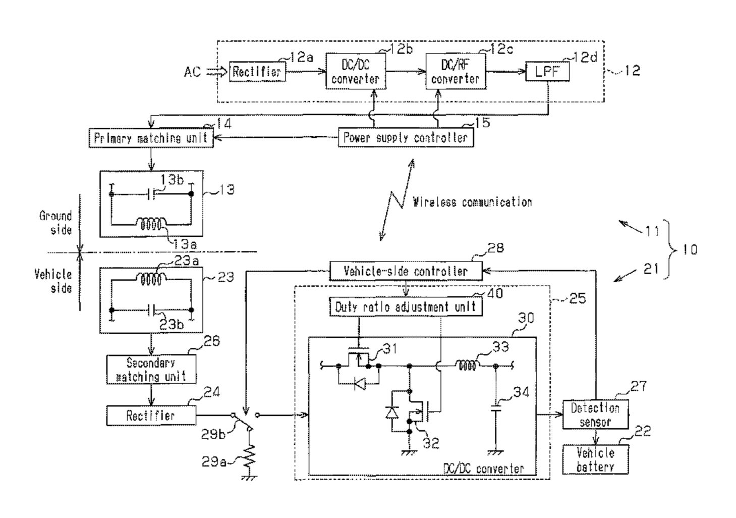
that performs a switching operation with a prescribed cycle. The charging device adjusts the duty ratio of the switching operation in accordance with the impedance of a load.
