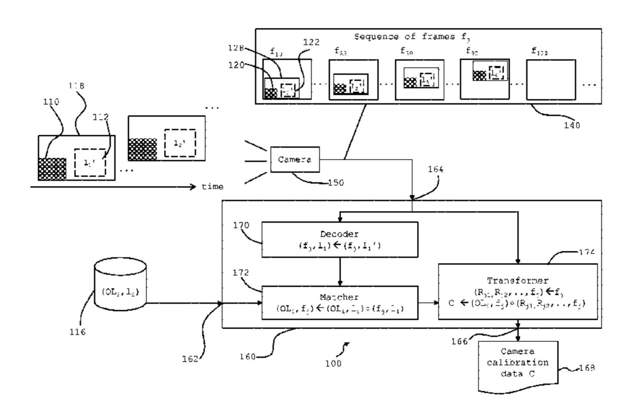
ture in the picture of the at least one frame. The camera calibration data of the at least one camera is determined by applying a geometric transformation (174) on the at least one reference point and its associated geopositional data of the moving object which is in the at least one frame.
