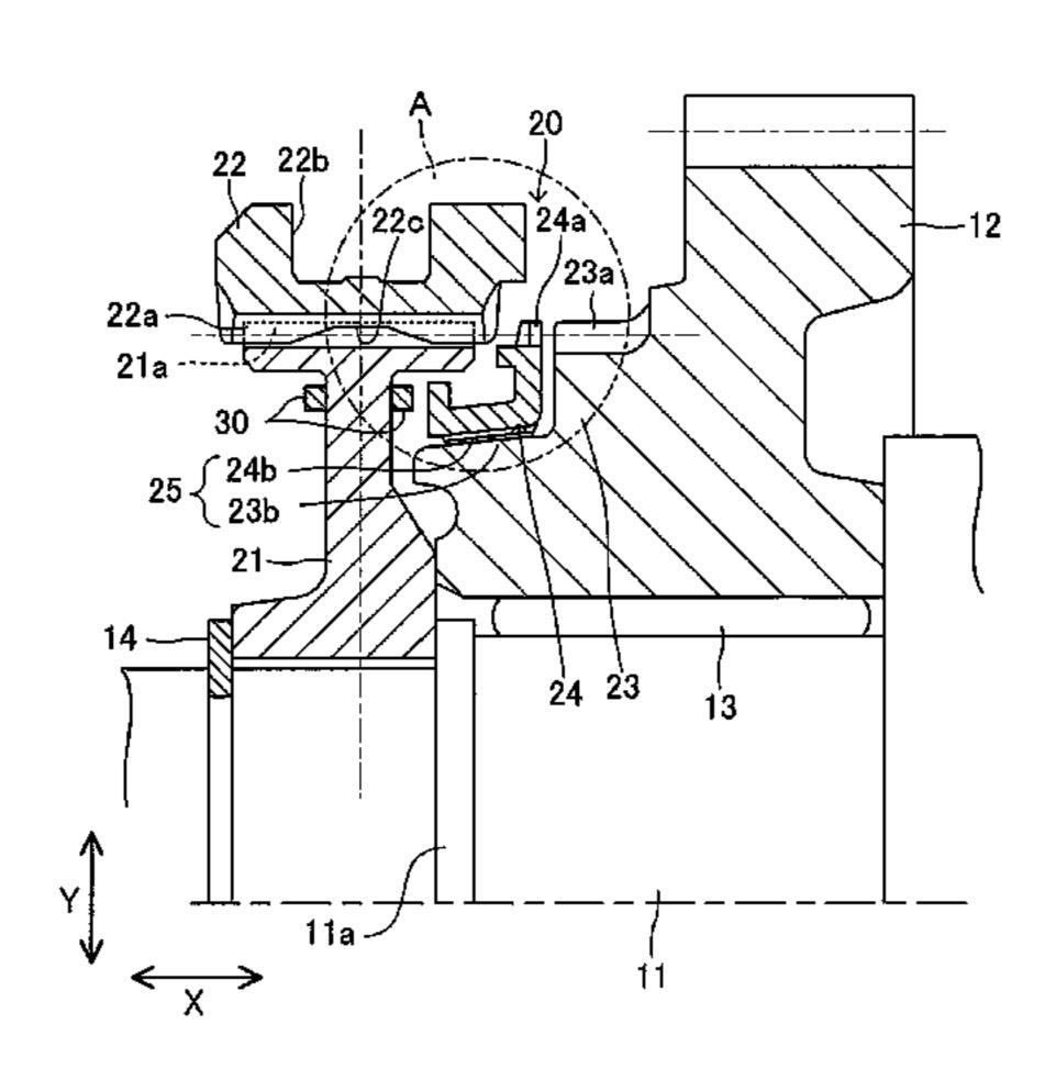
hub; and a radial protruding portion protruding from the ring body toward the clutch hub in a radial direction intersecting the axial direction to set a size of a radial clearance to be formed between the ring body and the clutch hub. The ring body, the axial protruding portion, and the radial protruding portion are formed integrally by metal stamping.
