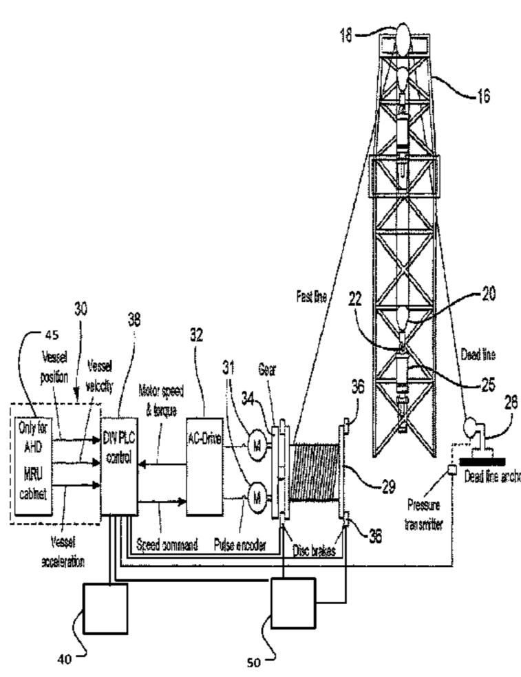
hoisting system is to perform an active heave compensation when operated in fixed-to-bottom mode; and wherein the hoisting system is adapted to prevent the emergency brakes from engaging.
