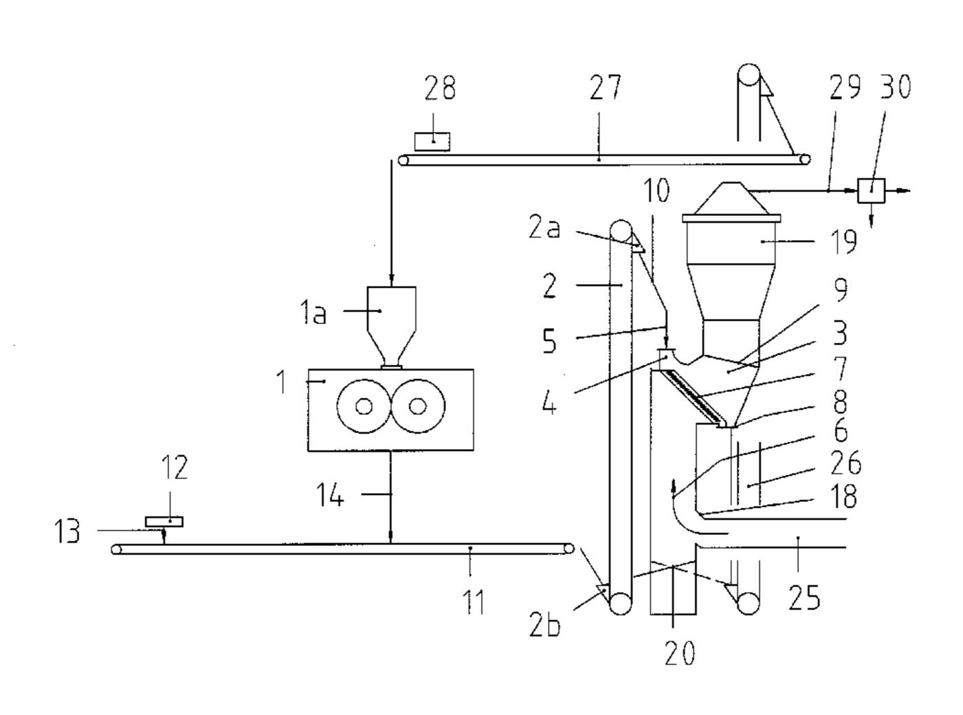
tion plate also permits sifting gas to pass there through from the lower to the upper sifting space. The static sifter also includes oversized material outlets disposed in each of the respective upper and lower sifting spaces.
