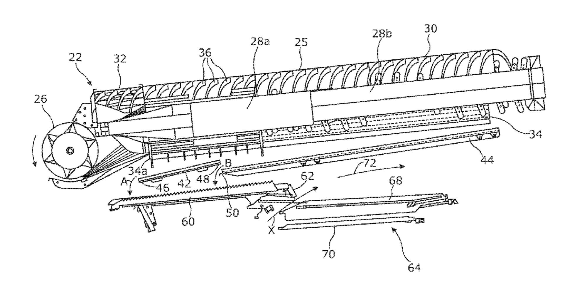
distance located behind the first region. The grain pan (60) serves to convey the collected grain in a rearward direction to a cleaning unit (64).
