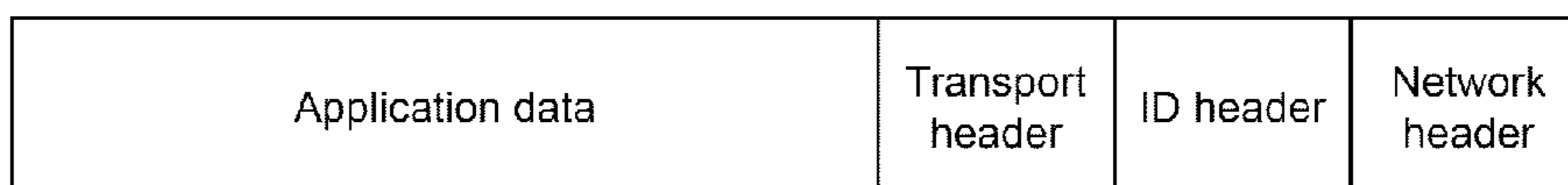
(a) Packet format with application data and transport, ID and network headers
