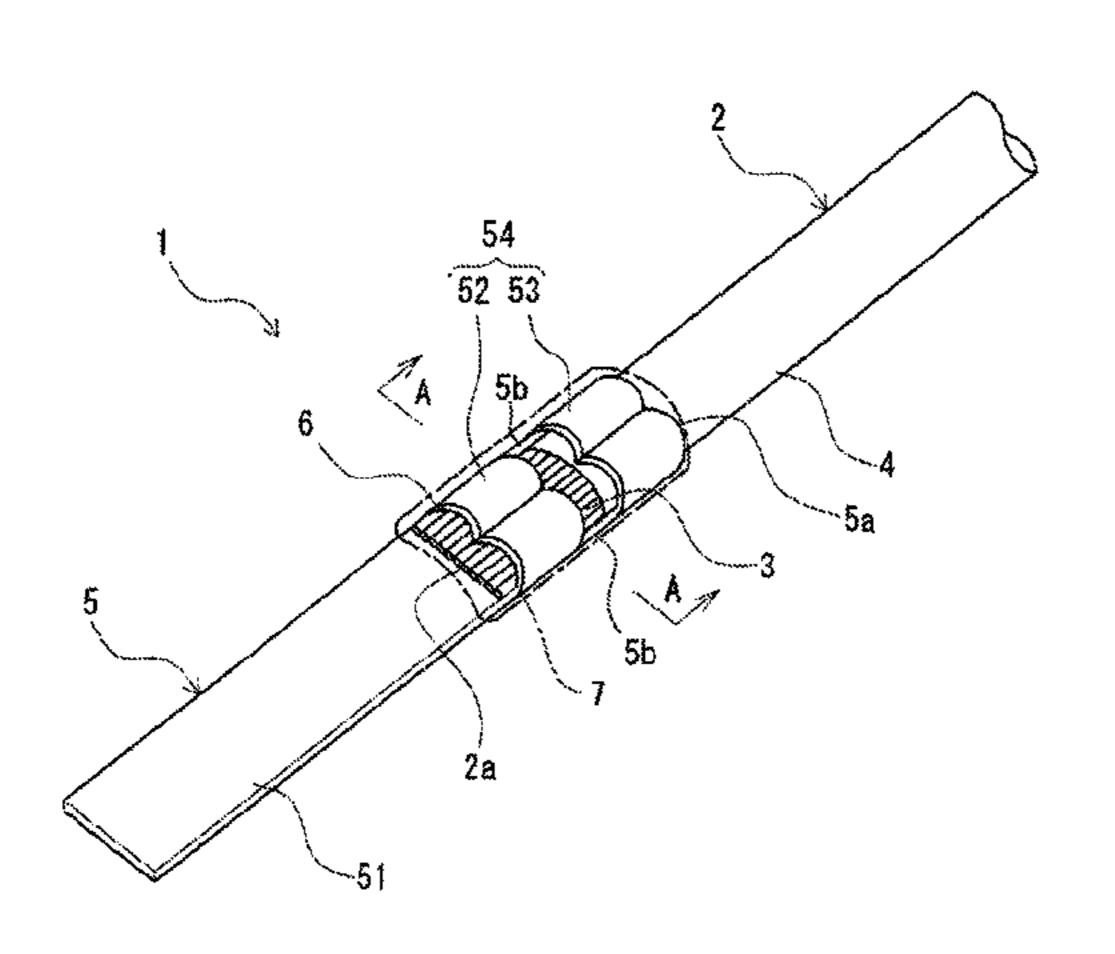
fitting, an electric wire conductor, and an electrical connection portion in which the terminal fitting and the electric wire conductor are electrically connected to each other. The terminal fitting has a surface to which processing oil adheres, and the electrical connection portion is covered with an anticorrosive agent containing an adhesive resin and an oil-adsorbing organic macromolecule to configure a terminated covered electric wire.
