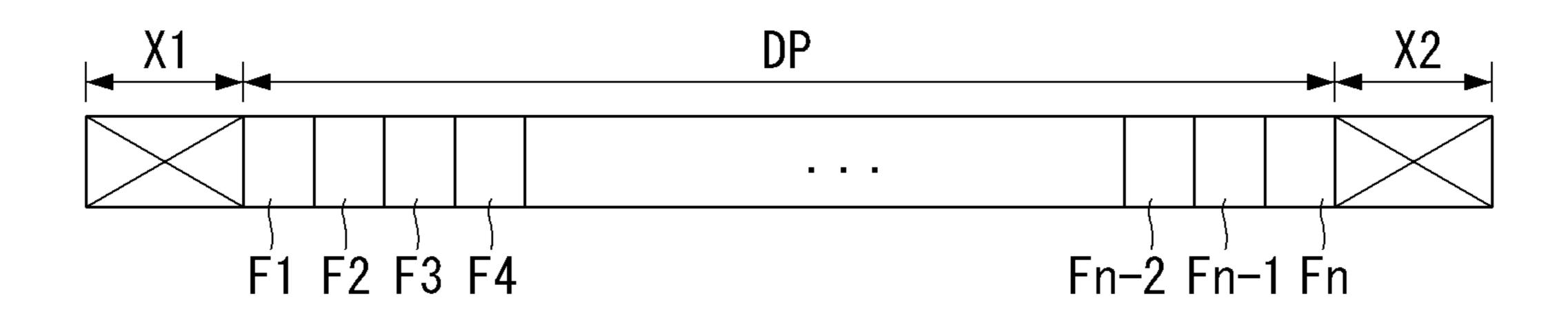
X1 or/and X2 : Vth external compensation DP:  $\mu$  internal compensation
