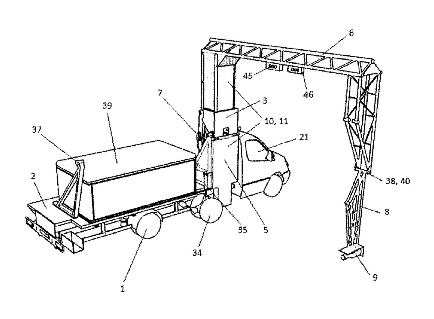
The system which implements the method presented earlier is constituted from a mobile scanning unit and a mobile control center which is positioned outside the exclusion area "a" which remotely command all the processes involved in the nonintrusive inspection.
