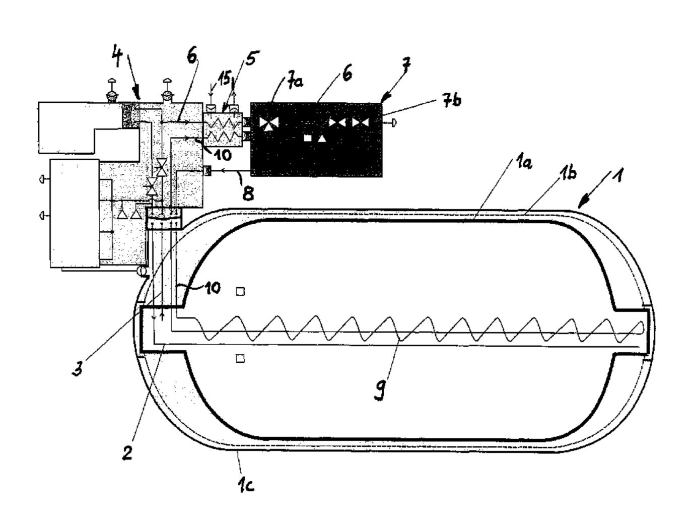
line caused upstream of the pressure regulating unit by switching the tank pressure regulating valve, a sufficient and continuous supply of hydrogen to the consumer at the pressure required is guaranteed.
