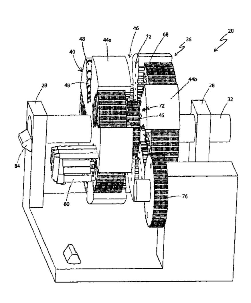
the key pulley segment is actuated to the engaging position and rotated into the contact zone, the corresponding mating features of the endless drive member engage the first set of mating features of the core pulley and the second set of mating features of the key pulley segment without the introduction of significant slack or tension.
