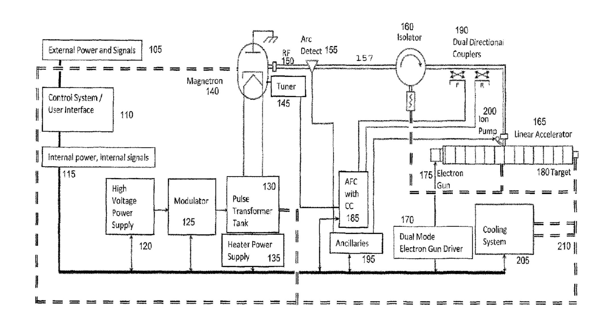
180 Target Linear Accelerator 165 Cooling System Dual Directional Pump Couplers 190 Electron Electron Gun Driver **5II** Dual Mode 175 Isolator 160 195 57 Ancillaries 185 with AFC Detect 155 Arc Tuner ₹ 150 145 130 Transformer Heater Power Pulse Supply Tank Modulator 125 105 120 internal signals Voltage and Signals Supply Power High Internal power, Control System External Power User Interface
