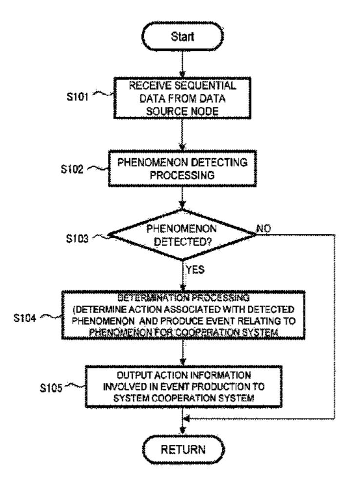
specifying a change attribute of contiguous time-series data pieces for each phenomenon leading to a particular result, and a determination section configured to extract action information associated with the particular result detected by the phenomenon detecting section to produce an event for a predetermined system based on action definition data previously specifying action information for each particular result.
