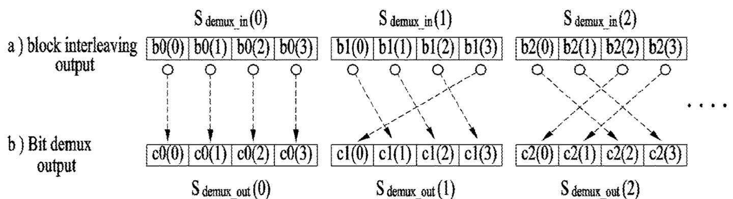
$$S_{\text{demux\_in}}(i) = \{b_i(0), b_i(1), b_i(2), \dots, b_i(\eta_{\text{MOD}} - 1)\},$$
