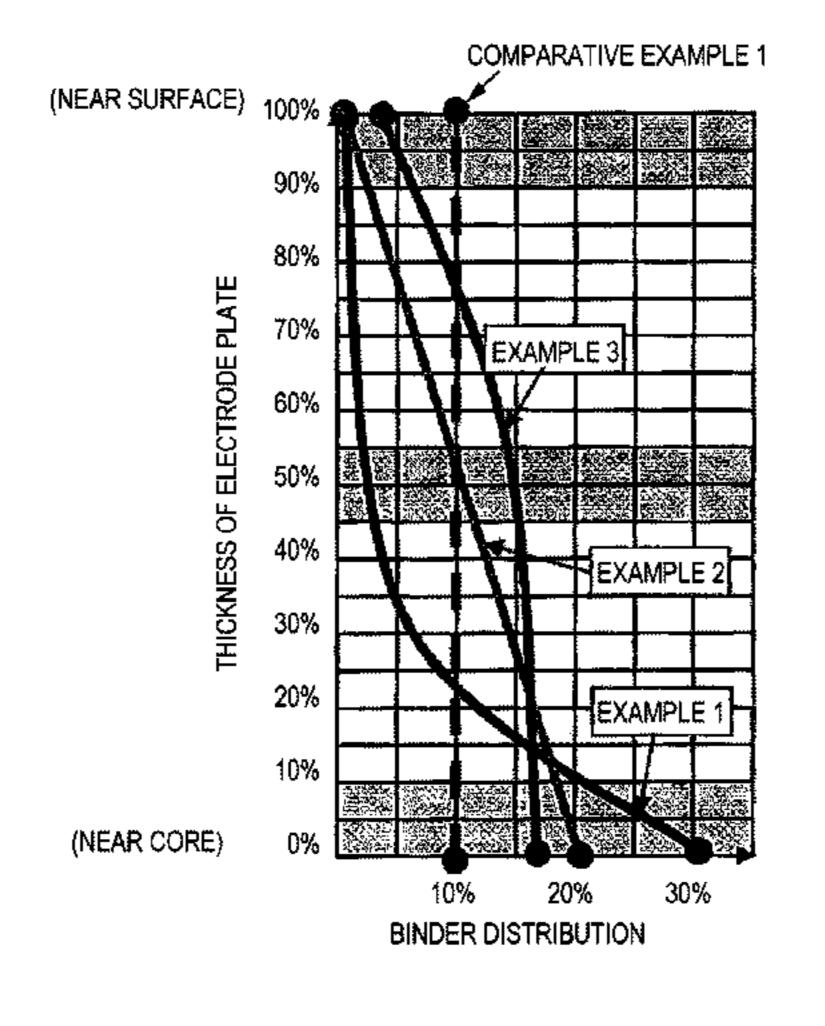
material layer to a position 100% of the thickness of the electrode active material layer from a surface of the electrode active material layer facing the core, with 10 being assigned to the amount of the binder present in the electrode active material layer per unit thickness if the binder is uniformly distributed in the electrode active material layer.
