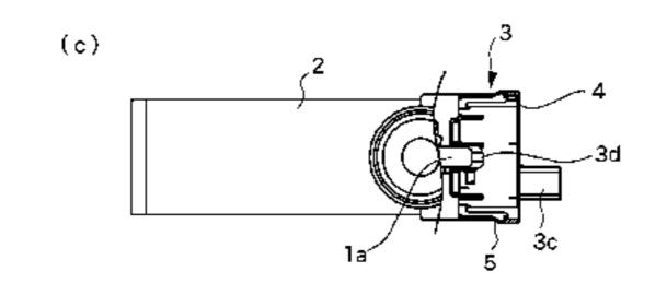
surfaces of the ignition switch 3 and the attachment recess 4 on the fitting start end side and the peripheral wall surfaces thereof on the fitting finish end side come into pressure contact with each other substantially simultaneously with each other when the depth of the fitting of the ignition switch 3 to the attachment recess 4 reaches a predetermined depth, to thereby reduce rattling in the radial direction.
