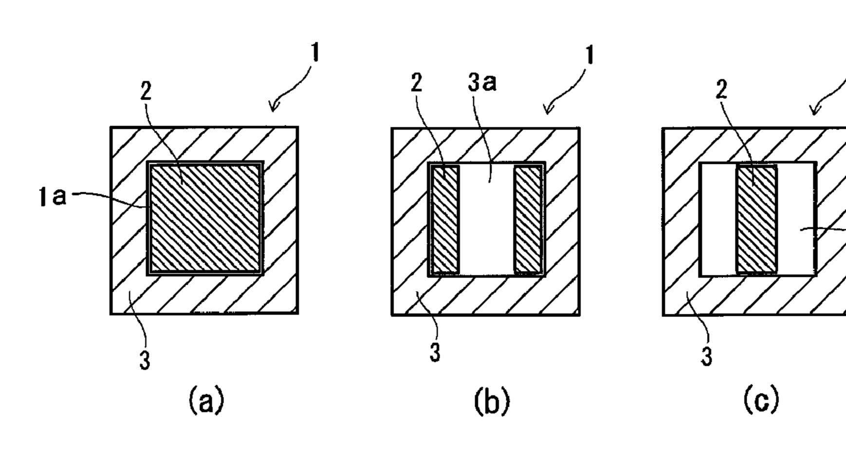
tion-molded magnetic body (3) or bonded thereto at a combining portion thereof to obtain the combined body. The combined body is composed of the injection-molded magnetic body (3) constituting a housing in which the compressed magnetic body (2) is disposed.
