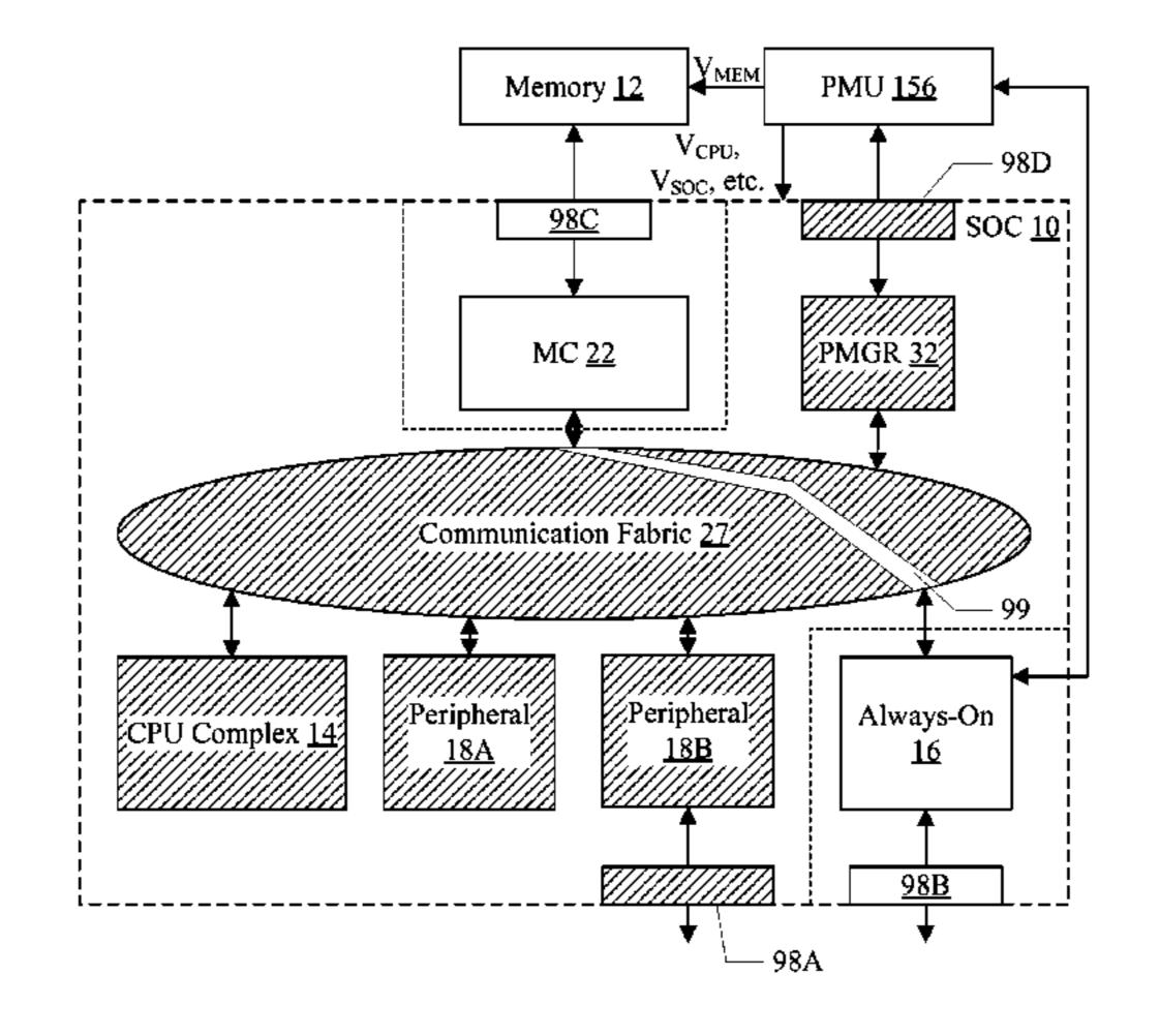
SOC and the path to the memory controller, in order to write the data to memory. The remainder of the SOC may remain powered down.
